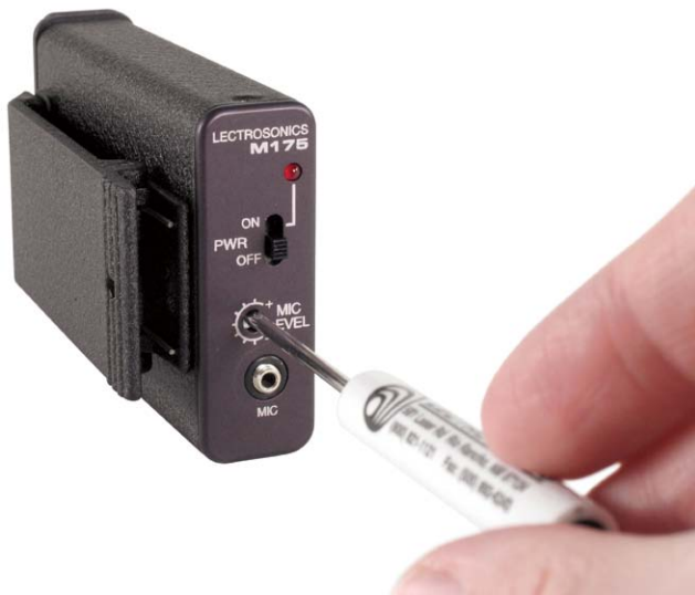
Figure 3 - Transmitter Gain Adjustment
